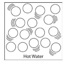
One example is the red alcohol inside the thin tube of a thermometer. When the thermometer is heated, the molecules of alcohol move faster. This faster motion competes with the attraction between the molecules which causes them to spread out a little. They have no where else to go so they move up the tube.
